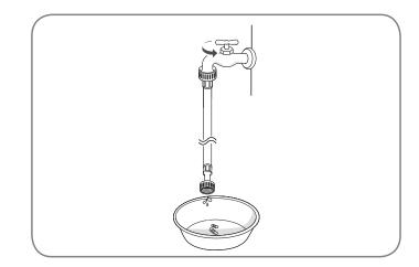
**3.** Always run a gallon or two of water through each inlet hose to flush dirt, scale and other debris out of the water lines. Doing so will help prevent future problems with clogged filter screens, and will also allow you to verify which hose is hot and which is cold.
